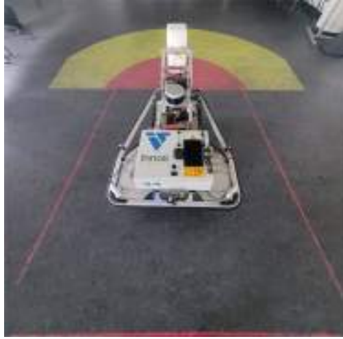
Fig. 2. The robot with the implemented visual communication tools for a violation of the stop zone. Laser lines on the sides and in the back, a projector towards the front.
