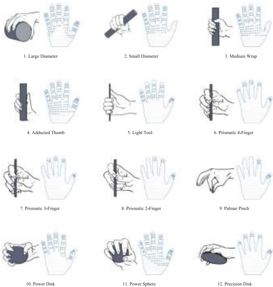
Fig. 2. Scatter hand map of touch point distribution on fingers and palm for various hand grasps.
