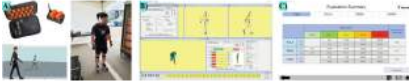
Fig. 1. IMU motion capture and locations of IMU motion sensor attachments (A), 3D-SSPP program (B), AutoChecklist program (C)
