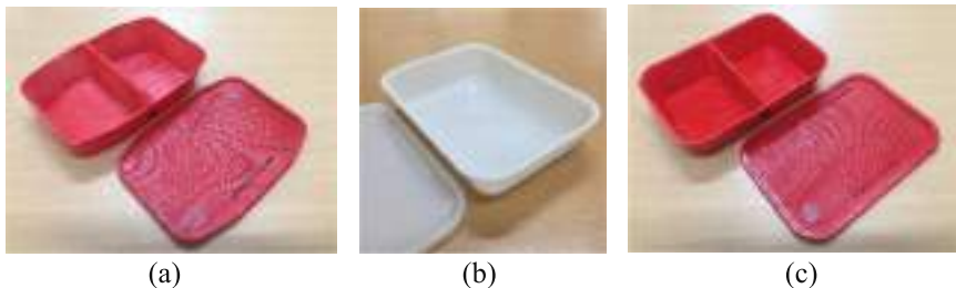
Fig. 2. Sample of plastic containers for the experiment: (a) angular, double, octagonal, with normal setup, (b) curved, single, rectangular, with explicit direction, angular, double, rectangular, with explicit direction
