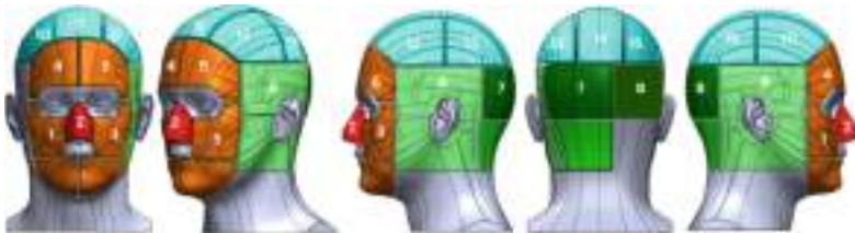
Fig. 2. PPS Tactile Head with Labeled Sensors
