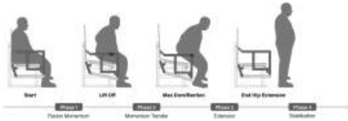
Fig. 2. The chair assists the user according to the stages of STS movement.
