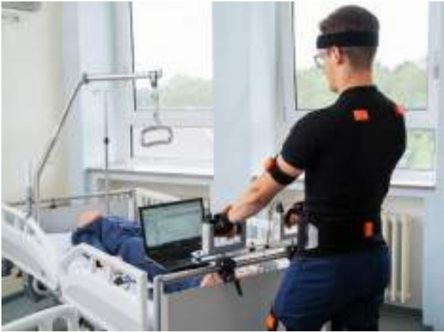
Fig. 1. Hospital bed with three-dimensional force transducers and caregiver with personal motion analysis system while maneuvering a bed out of the patient's room.
